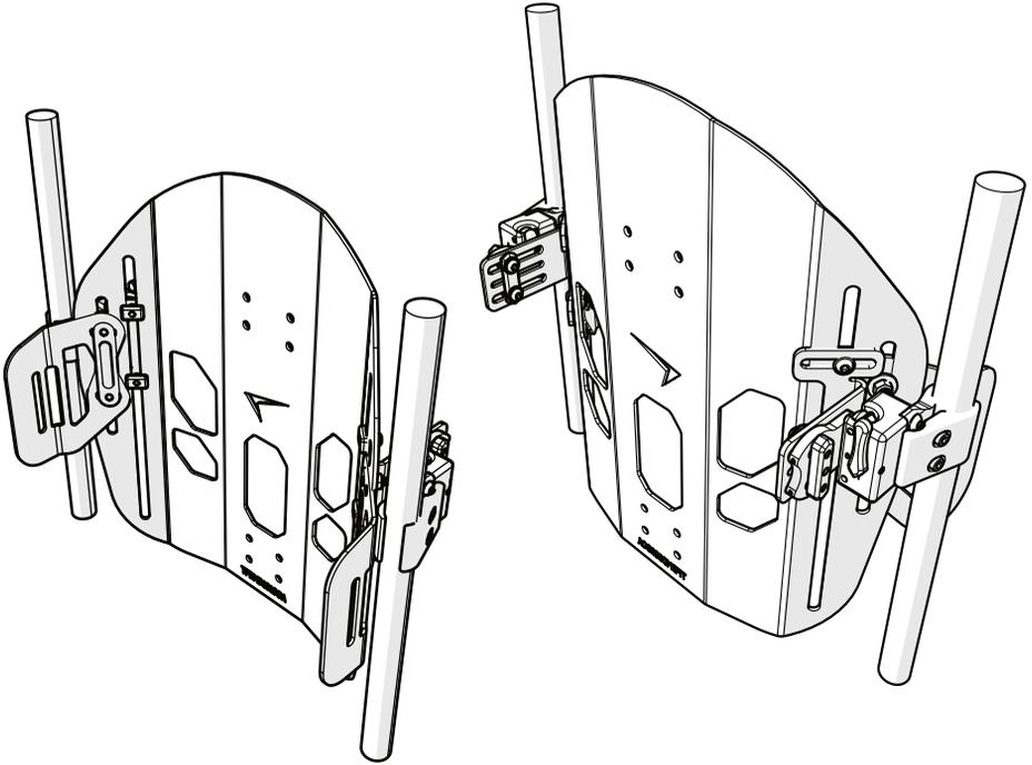
1. Install the **Fliplock** hardware to the back shell. See page 3, "*Mounting the Hardware to the Back Shell*" in the TFB Simple Solutions Removable Hardware Manual.
