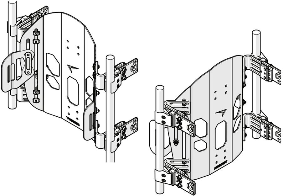
1. 4-point Heavy Duty installation utilizes the **Simple Solutions Stability** hardware in both upper and lower positions on the back shell. Install the hardware in these positions. See page 3, "*Mounting the Hardware to the Back Shell*" in the TFB Simple Solutions Fixed Hardware Manual.
