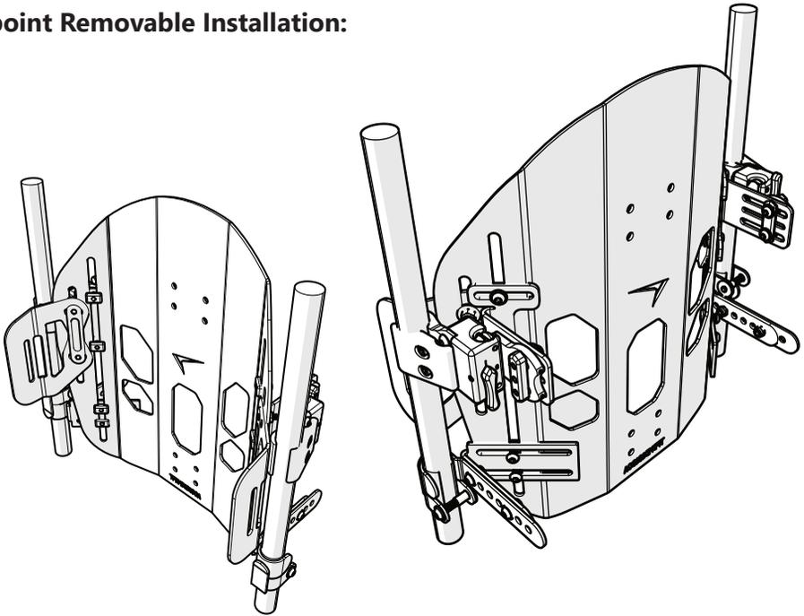
1. 4-point removable installation requires the **FlipLock** hardware in the upper position of the back shell, and the **J&L** hardware in the lower position. Install the hardware in these positions. See page 3, "*Mounting the Hardware to the Back Shell*" and page 5, "*Mounting the J&L Hardware*" in the TFB Simple Solutions Removable Hardware Manual.
