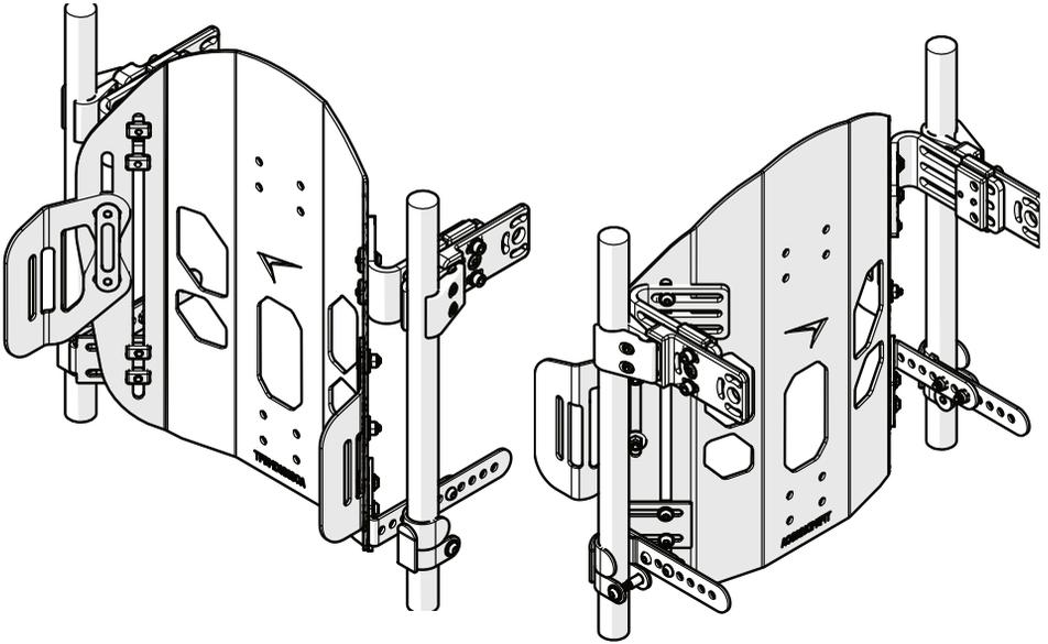
1. 4-point fixed installation requires the **Simple Solutions Stability** hardware mounted in the upper position of the back shell, and the **J&L** hardware in the lower position. Install the hardware in these positions. See page 3, "*Mounting the Hardware to the Back Shell*", and page 5, "*Mounting the J&L Hardware*" in the TFB Simple Solutions Fixed Hardware Manual.
