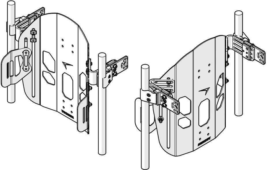
1. Install the **Simple Solutions Stability** hardware to the back shell. See page 3, "*Mounting the Hardware to the Back Shell*", in the TFB Simple Solutions Fixed Hardware Manual.
